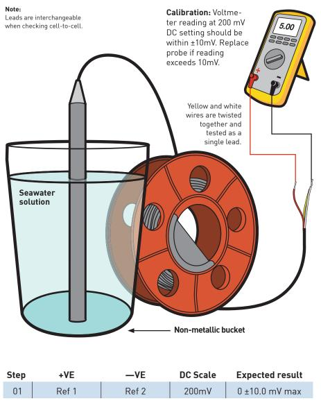
Note: To avoid damaging the cable, do not invert the DC-II™ when placing it in the bucket.
